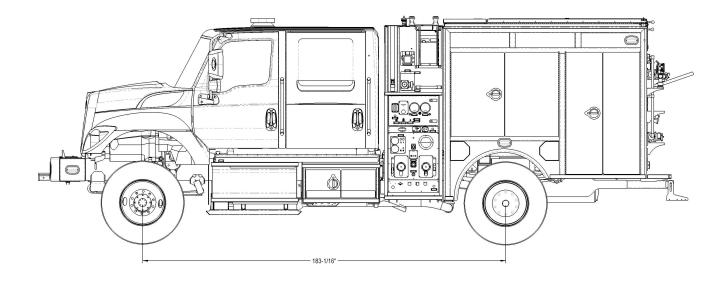
International® HV507, 4 Door, Single Axle, 4x4 Cummins® ISL 350 HP Engine Allison® 3000 Transmission Darley® JMP 500, 2-Stage Pump Darley® 1½ AGE Auxiliary Pump 24 HP Kubota® D902 Diesel, Water Cooled Hannay® Hose Reel with Electric Rewind Welded Steel Body Construction
