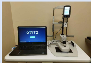
OVITZ xwave system used for aberrometry measurement and wavefront-guided lens design
