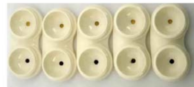
Fig. 4. Microbiosensor in a contact lens case with the bottom blue colour indicating microbial contamination [525].
