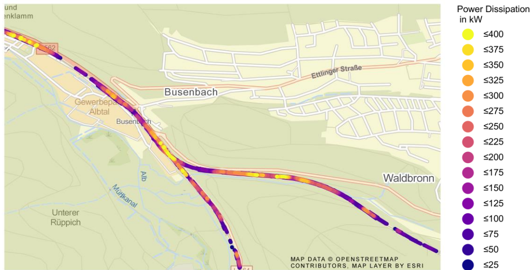
Figure 3: Power dissipation at the braking resistor along the track
