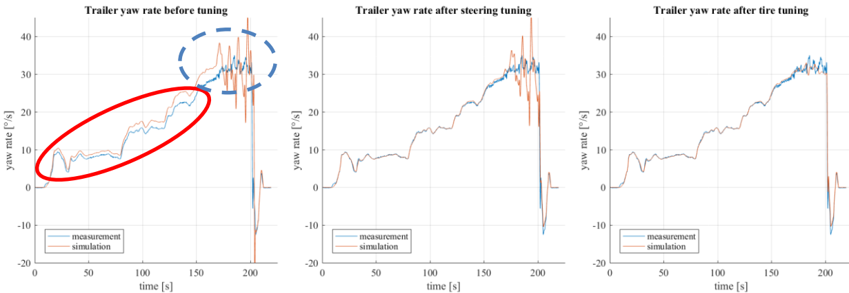
Figure 12: yaw rate during constant radius circle maneuver, before and after tuning
