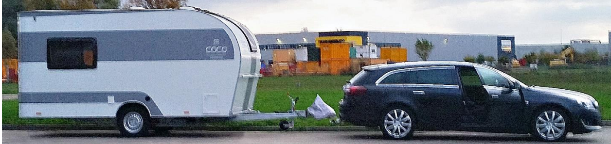
Figure 8: Actual test-drive setup, hitch force measurement hardware hidden under cap
