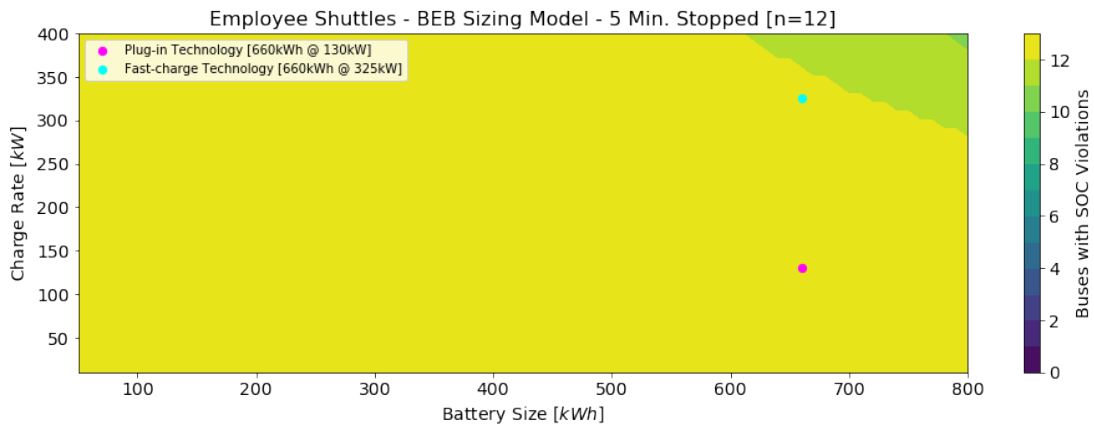
Figure 12: Employee shuttle model results for charging when the buses is stopped for 5 minutes or longer
