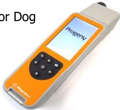
Handheld Raman Spectrometer (2015)
